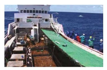
Picture 23. Skipjack flow by gravity to conveyor belt that transports fish directly to refrigerated brine well (Photo: T. Kawamoto)
