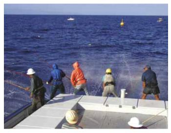
Picture 20. Landing area for poled tuna covered with a smooth vinyl tarp wetted with seawater (Photo: D. Itano)
